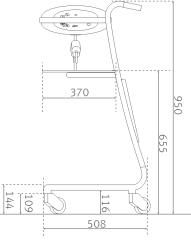
Drawings and technical specification refer to horisontal Luna with 2-point spreader bar.
